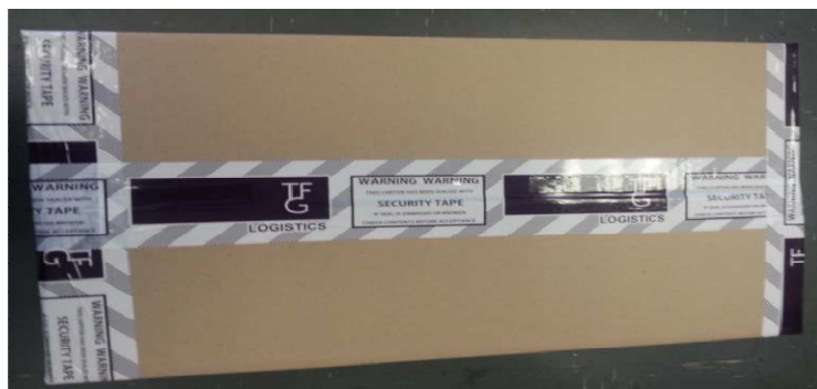
Fig 7.1: Carton to be sealed in H-Pattern on both top and bottom sides
